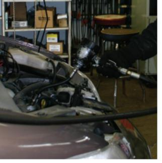
SAE viscosity grade ratings for commonly used motor oils typically range from zero up to 50. A "W" after the number stands for "Winter" grade oil, and represents the oil's viscosity at subzero temperatures. Low viscosity motor oils that pour easily at low temperatures typically have a "5W" rating. There are also 10W, 15W and 20W grade motor oils.
